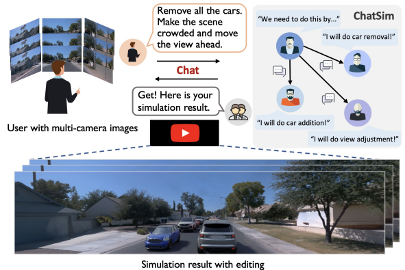
Figure 1. ChatSim enables the editing of photo-realistic 3D driving scene simulations via language commands.
