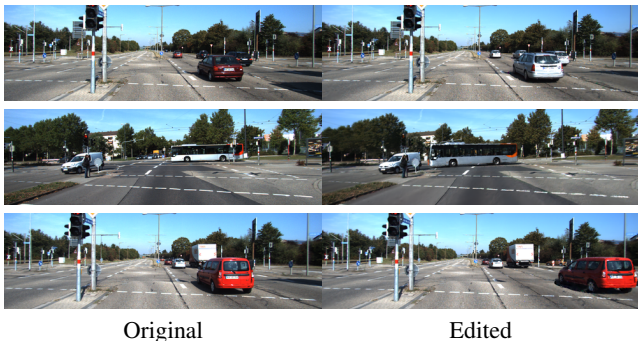
Figure 8. Scene Editing on KITTI. Our decomposed scene representation enables replacing dynamic objects (1st row) and moving dynamic objects around (2nd & 3rd rows).
