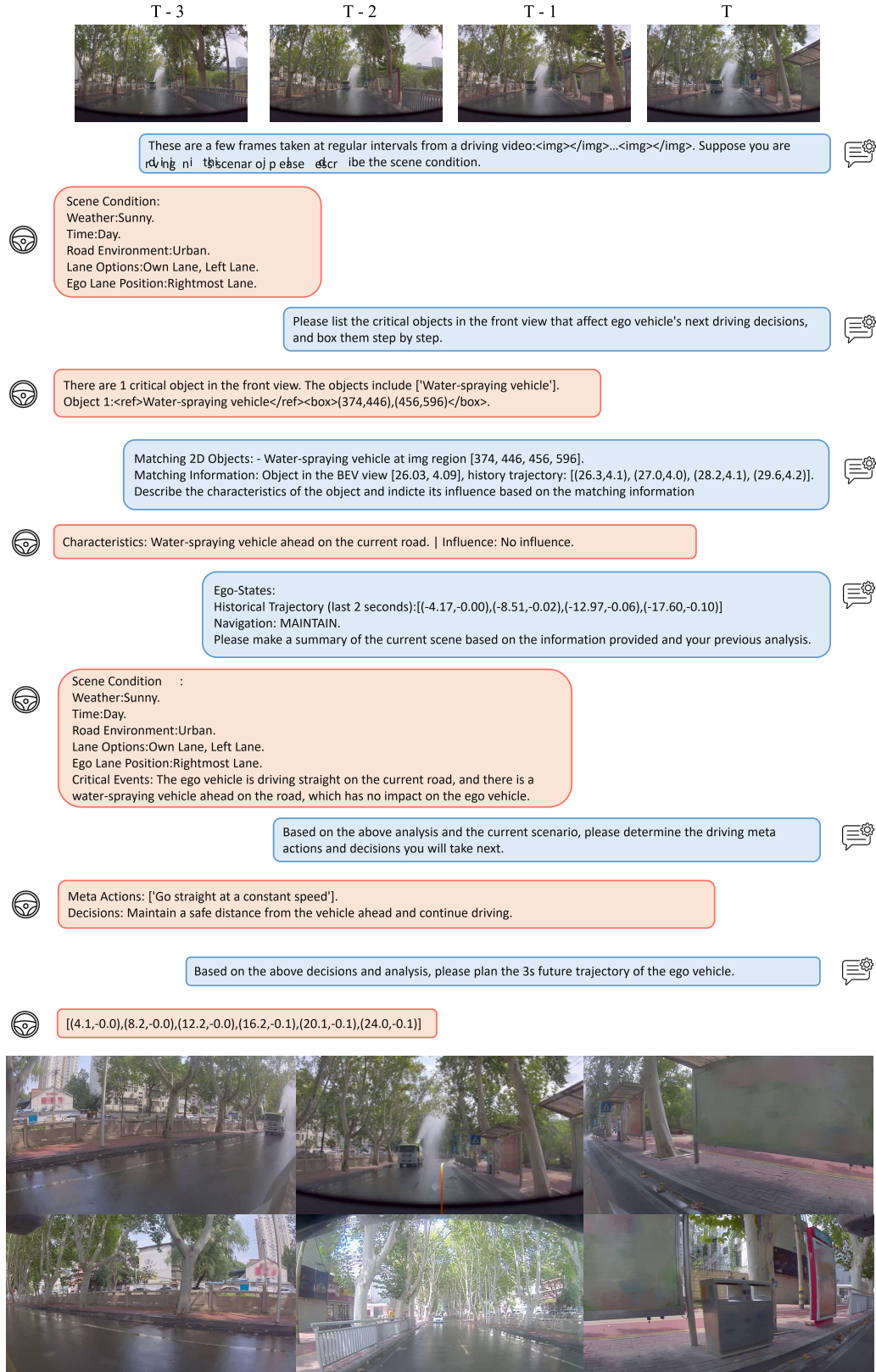
Figure 15. Visualization of DriveVLM's output. DriveVLM has identified the type of the unconventional vehicle ahead.
