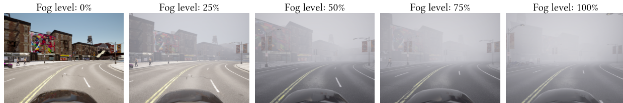
Figure 4: Carla simulation sample image across fog intensities of 0%, 25%, 50%, 75%, and 100%. The visibility of the road incrementally reduces as the fog intensity increases.
