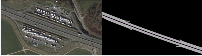
Fig. 4. Comparison of Google Maps satellite imagery against our generated OpenDRIVE example. The main highway is based on the calculation of the reference line, while the off- and on-ramp are derived from OpenStreetMap.
