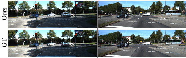
Figure 6. Qualitative results on KITTI. With only 25% of views (approx. 15-20) for training, we can still synthesize sharp and realistic novel views with dynamic objects rendered at high quality.
